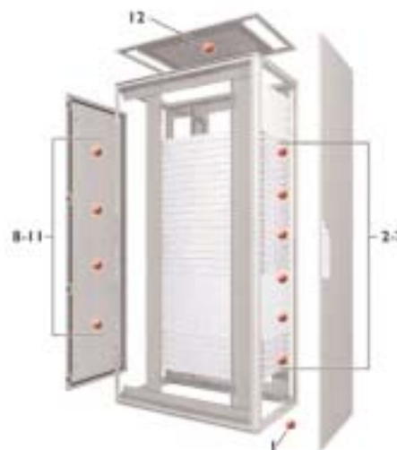
Figure 5 ■ – denotes thermal probe locations
