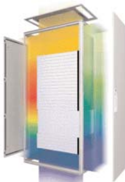
Figure 7B: The thermal drawing represents the heat dissipation from test 18 with solid front and rear door with roof fan
