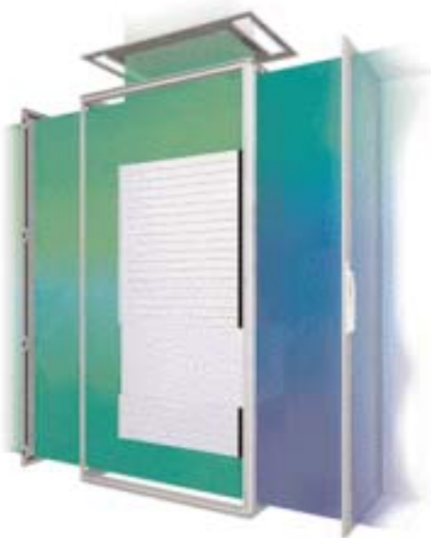
Figure 7A: This thermal drawing represents the heat dissipation for test 3 with perforated front and rear door and vented roof
