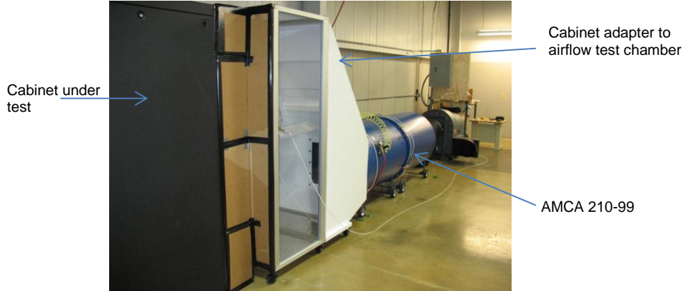
Figure 1. Airflow testing setup. From left to right: the cabinet under test (black) cardboard adapter, cabinet adapter to airflow test chamber (white) and AMCA 210-99 (blue).
