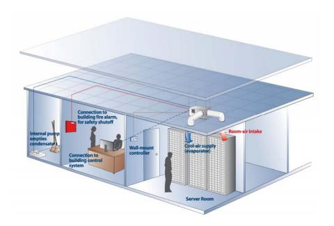
Self-contained, ceiling-mount air conditioners easily fit into the crawl space above server room and closets. Self-contained, ceiling-mount conditioners are most notable for their low cost and quick, easy installation. Unless there are special circumstances, a typical installation usually takes two installers working together only about four hours.
